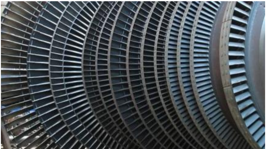
Figure 3. Steam Turbine Rotor
